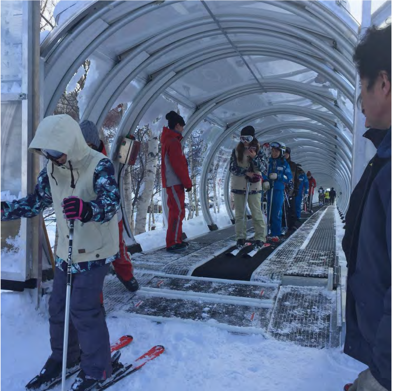
2017 – Teine (Japan) – Length 116 m – Band width 600 mm
