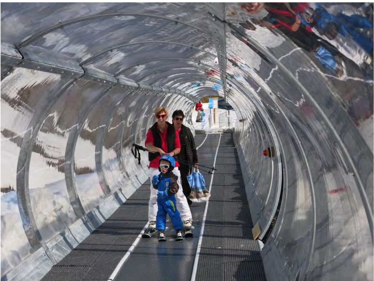
2014 – Châtel (France) – Conveyor “Pré la Joux” – Length 220 m – Band width 760 mm
